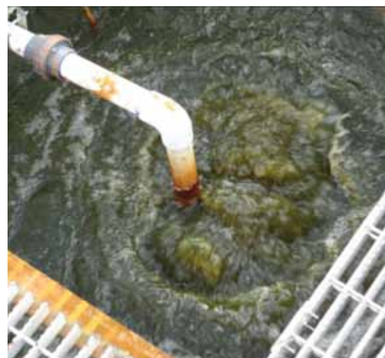
Figure 8. (above right) Manor "A-Mixer" used to enhance lime mixing and dissolution.
